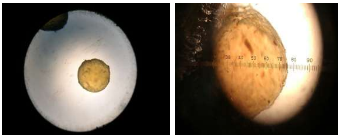
Figure 1: Optical photograph of microsphere with & without eyepiece micrometer
