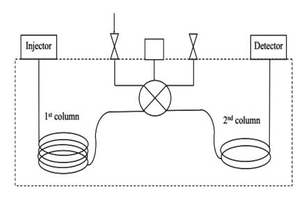
Figure 5: Schematic diagram of GC×GC instrument with a valve-type modulator.
