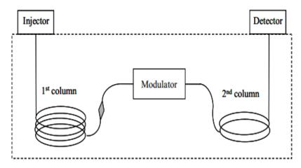
Figure 1: Schematic diagram of GC×GC apparatus.
