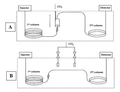
Figure 4: Schematic diagram of GC×GC instrument with cryogenic modulators: (A) longitudinally modulated cryogenic system (LMCS) (B) dual-jet modulator
