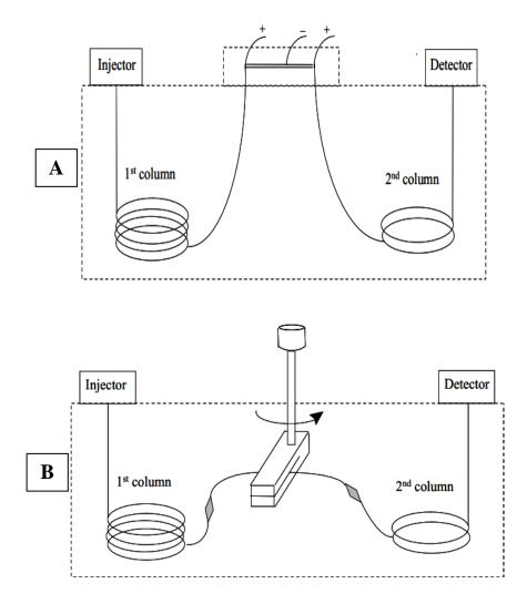
Figure 3: Schematic diagram of GC×GC instrument with thermal modulators: (A) two-stage thermal modulator and (B) Sweeper.
