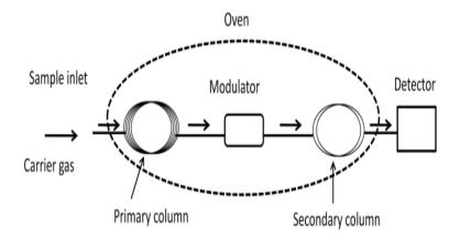
Figure 2: Schematic diagram of GC×GC apparatus.
