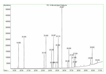
Fig. 1. GC-MS chromatogram of standard mixture of 13 pesticides and its metabolites at 2 ppm level.
