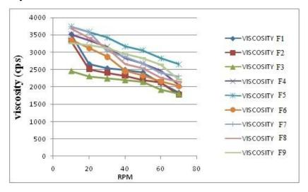
Fig. 1: Comparison of angular viscosities of formulations
