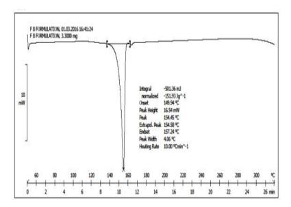
Fig 12: DSC graph of simvastatin drug loaded formulation (8)
