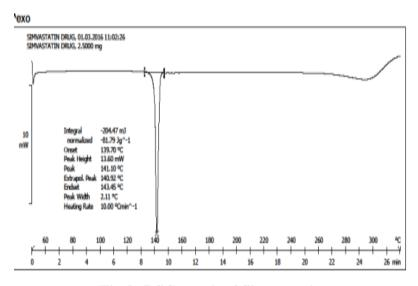
Fig 8: DSC graph of Simvastatin
