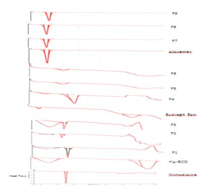
Figure 4: DSC of pure Nimodipine and its formulations prepared by Solid dispersion (SD)
