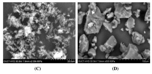
Fig 9: Scanning Electron Microscopy of (A) Febuxostat, (B) soluplus, (C) Physical mixture (FBXS2), (D) Solid dispersion (FBXS2).
