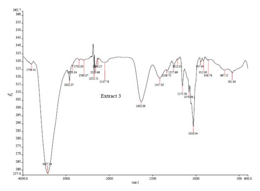
Figure 5: FT-IR spectra of lantana camara extract with silver nanoparticle
