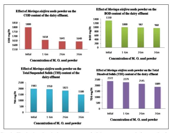
Graph II physico-chemical parameters of dairy wastewater before and after treatment with M. oleifera seeds powder
