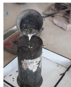
Figure 3 B: Molten Yashada Poured to pitara Yantra.
