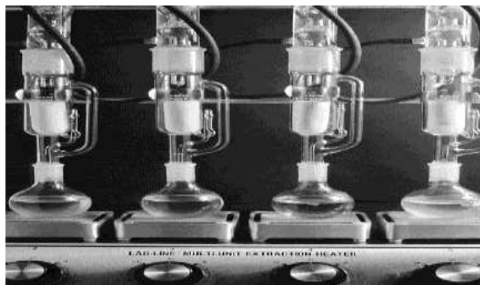
Fig. 2: Demonstration of a Soxhlet apparatus.
