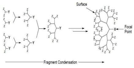
Fig. (b): Convergent synthesis of dendrimer. [9]
