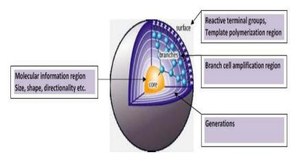
Fig. 1: The Dendrimer Structure.
