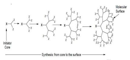
Fig. (a): Divergent synthesis of dendrimer. [9]
