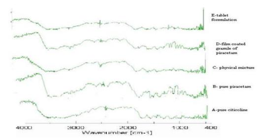
Fig. 3: Comparative IR spectral data A) Pure Citicoline, B) Pure Piracetam, C) Physical Mixture D) film coated granules of Piracetam, E) Tablet formulation.
