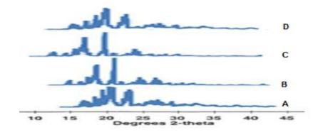
Fig. 6: Comparative XRD spectral data A) Pure Citicoline, B) Pure Piracetam, C) film coated granules of Piracetam, D) Tablet formulation.
