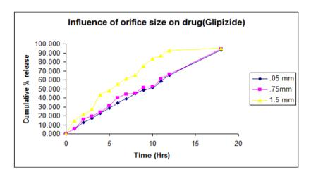
Figure. 4 (b): Influence of orifice diameter on Glipizide release profile.
