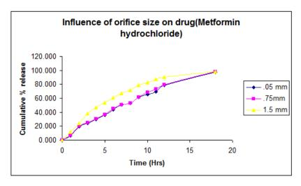
Figure. 4 (a): Influence of orifice diameter on Metformin HCl release profile.
