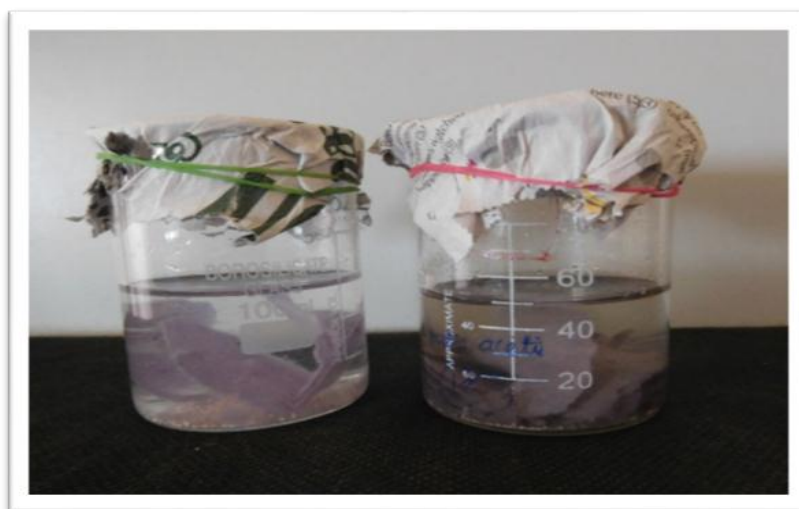
Fig. 3. Mycelial mat residues treated in acetic acid for the separation of Chitin / chitosan.
