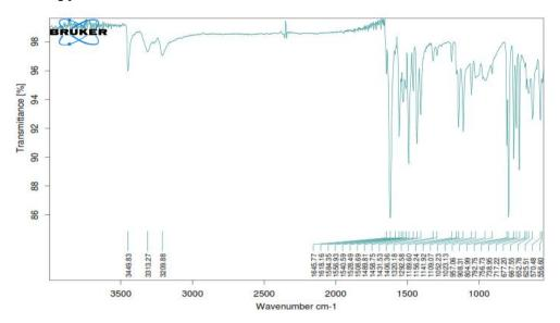
Figure 5: FTIR Spectrum of pure Ondesartan hydrochloride drug.
