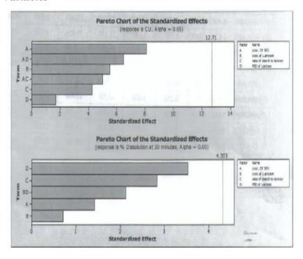
A Pareto chart showing the effect of core tablet formulation process variables on Tablet Content Uniformity (%) and % dissolution at 30 minutes **Pereto Chart of Formulation variables on Tablets Content Uniformity and % Dissolution at 30 minutes.** The estimated effect for each individual terms are presented in table 7 & 8 and figre-1.
