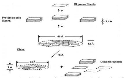
Fig. 4: Planar aggregates of 6–10 nm melanin protomolecules form sheet-like structures approximately 11  $\rm \mathring{A}$  thick. [48]
