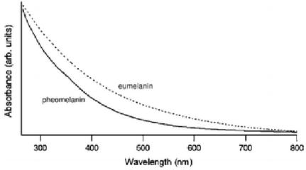
Fig. 5: The broad-band optical absorption spectrum of eumelanin and pheomelanin in the UV-visible region.<sup>[52]</sup>
