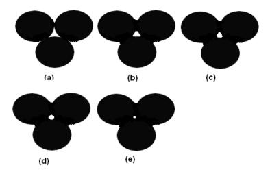
Figure 2: Three-sphere sintering model. (a) Original points of contact; (b) Neck growth; (c) and (d) Pore rounding; (e) Pore shrinkage.
