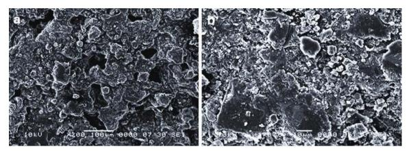
Figure 3: Scanning electron microscope images of a) unsintered and b) sintered tablet surfaces.
