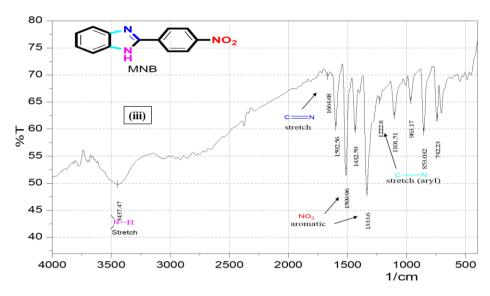
Figure-1: FTIR spectra of (i) MCB produced (a) in DMF, (b) in Toluene, and (c) in Dioxane solvent; (ii) MHB produced (a) Dioxane, (b) Toluene; (iii) MNB in Toluene.
