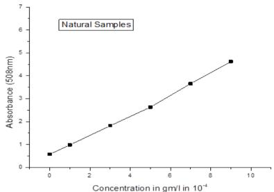
Figure 2: Concentration curve for Natural Samples for AAS
