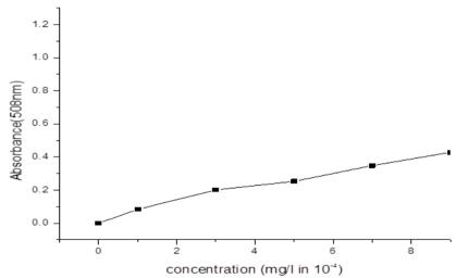
Figure-1 Absorbance -Fe Concentration curve
