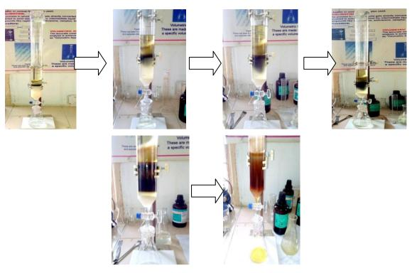
Fig 2: Separation by Column Chromatography.
