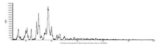
Fig 4: X-Ray Diffraction study of nateglinde pure drug.
