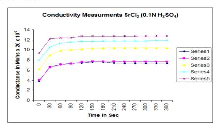
It has been observed that with the increase of concentration of solution the conductance of solution also increases and then become constant it is because of mobility of ions increases during the formation of strontium sulphate and becomes constant because the precipitate has been formed.
