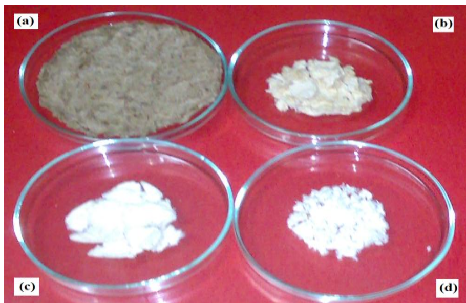
Fig.A: Microcrystalline cellulose extracted from banana fiber using steam explosion method where a) steam exploded fiber b) bleached fiber c) acid treated fiber and d) mechanically treated fiber.
