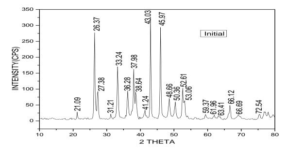
Powder X-ray diffraction of the final compound
