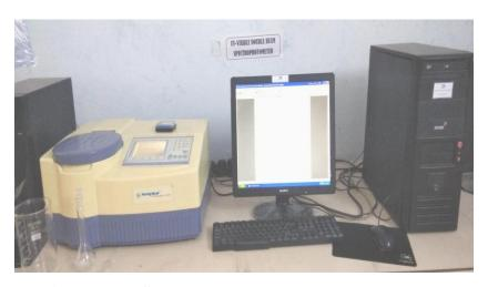
Fig.1: UV-VISIBLE double beam spectrophotometer.
