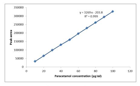
Figure [3]: Calibration curve for paracetamol.
