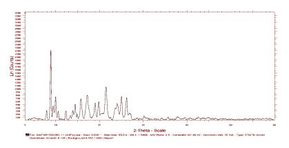
Fig. 5: X-ray Diffractogram of Fe(III) complex.
