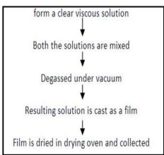
Fig. 1: Solvent casting apparatus and procedure. [5]
