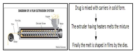
Fig. 2: Film extrusion apparatus and procedure. [5]
