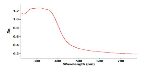
Fig. 1: UV-Vis spectrum of synthesized CeNPs.
