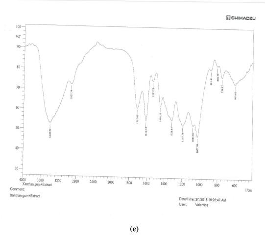
Figure 1: FT-IR spectra performed using FTIR Spectrophotometer (IR-470; Shimadzu, Japan), scanned over the range of 4000 to 400 cm-1, Infrared spectroscopic analysis was done for the powder of *Q. infectoria* galls, polymers (Carbopol 940 and Xanthan gum), physical mixture of drug and polymers 1:1.
