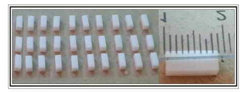
Figure 3: Zirconia substructures samples.
