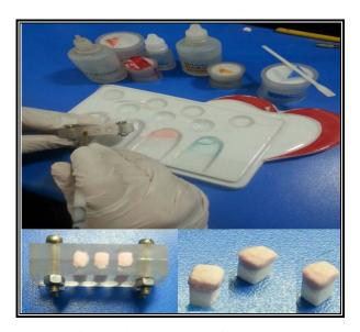
Figure 4: Build up of ceramic.
