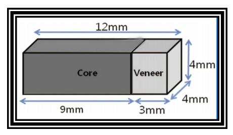
Figure 1: Final dimensions of the specimen.
