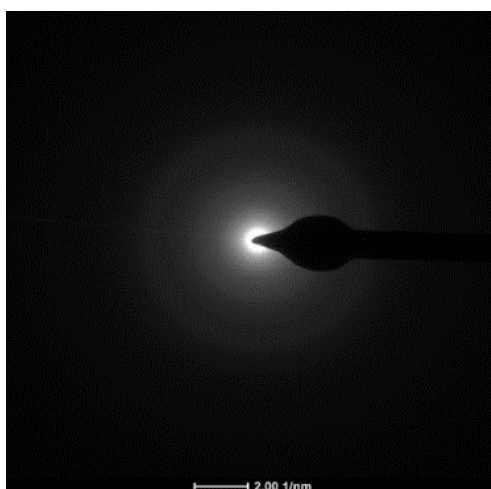
Figure 4: TEM Diffraction pattern of copper nanoparticles from \text{CuSO}_4 salt.
