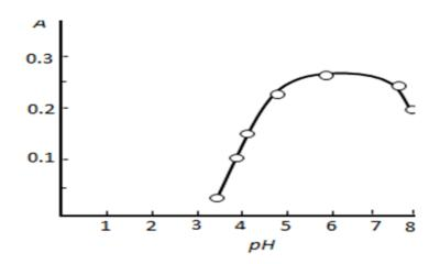
Fig. 2: Absorbance of mixed-ligand complexes as a function of the pH of the aqueous phase.  $C_{Ni}=2.035 \cdot 10^{-5}$  M.  $C_{DTEP}=C_{BPhen}=1.0 \times 10^{-3}$  M, 440 nm, l=0.5 cm.
