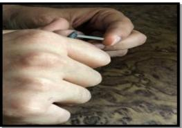
Figure (5): (a) divesting after casting, (b) smoothing the metal sample.
