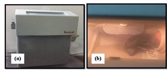
Figure (6): (a) The sand blast device, (b) A metal sample under sand blasting.
