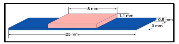
Figure (1): The prepared metal-ceramic sample dimensions.
