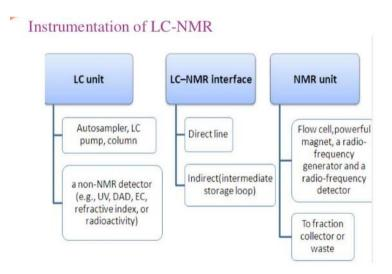
Figure. 4.2.: Instrumentation of LC-NMR.
