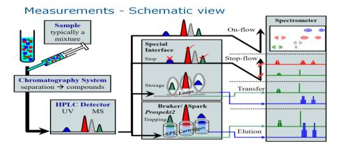
Figure. 5.2: Measurements Schematic view.
