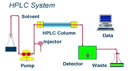
Figure. 4.1: Instrumentation of HPLC.
