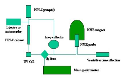
Fig. 1: Schematic repersentation of LC-NMR.
