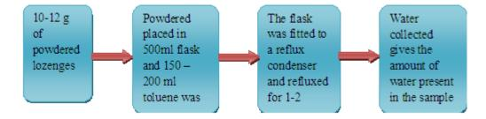
Azeotropic distillation method for moisture analysis.
