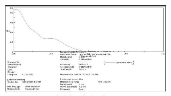
Fig. 2: Determination of  $\lambda$ max.
