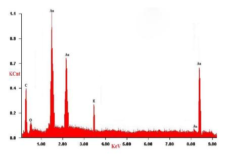
Figure 4: Au-NPs – EDS Analysis.
