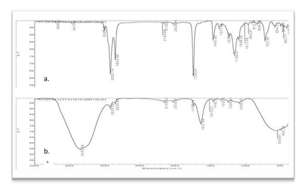
Fig1:a. FTIR of neem oil; B. FTIR on neem oil + lemon grass oil.
