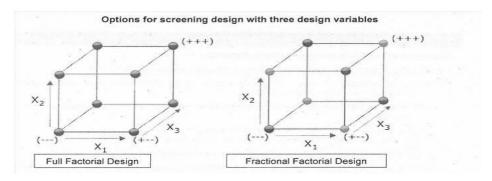
Figure 1: Description of full factorial design and fractional factorial design.
