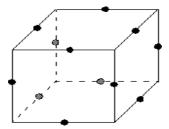
Figure 2: Three-factor Box-Behnken design.
