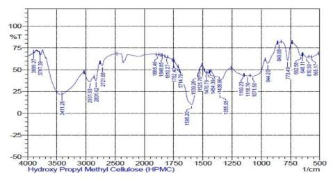
Fig. 2: Shows FTIR Peaks of Various Functional Groups of Polymer HPMC.
