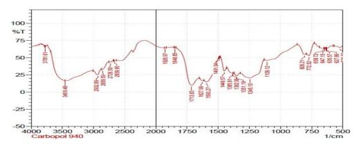
Fig. 3: Shows FTIR Peaks of Various Functional groups of Polymer CARBOPOL-940.
