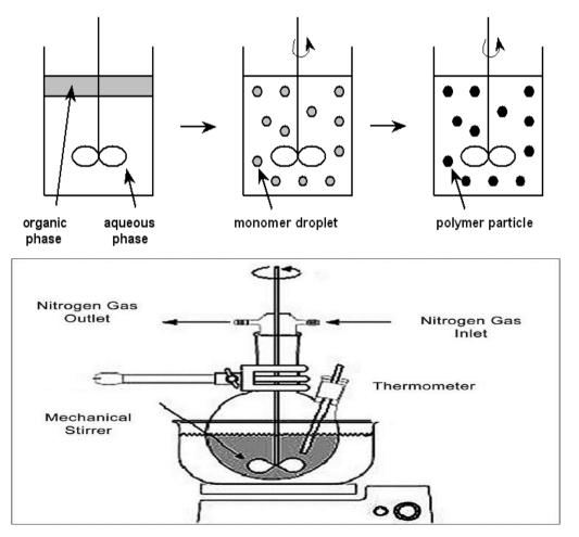
Figure 2: Liquid-liquid suspension polymerization.
