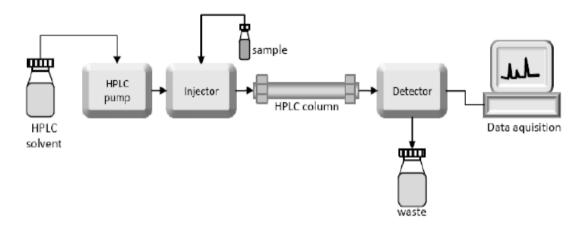
Figure 1: Block diagram of HPLC.
