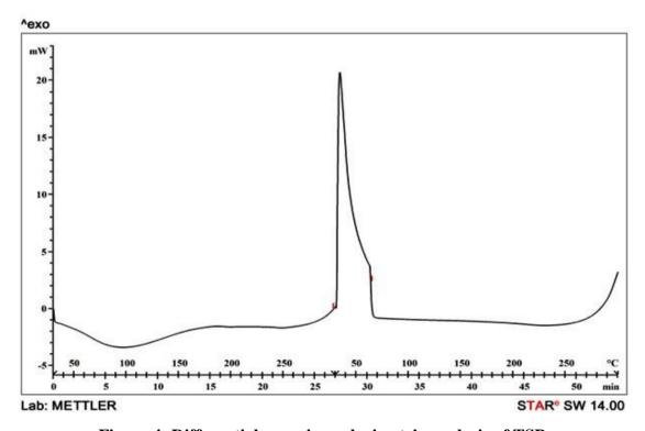
Figure 4: Differential scanning calorimetric analysis of TSP.
