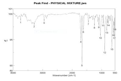
Figure.2: FT-IR Spectroscopy of physical mixture.
