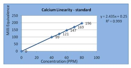
Fig. 2: Linearity of Calcium standard.
