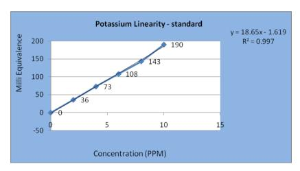
Fig 6: Linearity of Potassium Standard.
