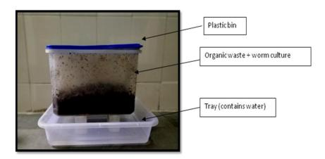
Figure 1: Small scale setup of vermicomposting unit.
