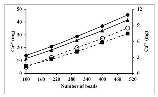
Figure 5: Number of beads in function of  $Ca^{2+}$  consumed for SG800 (10 g/L) polymerized at 30°C (dashed lines) and 40°C (solid lines) with  $CaCl_2$  0.1M [30°C: (o); 40°C: ( $\triangle$ )] and 0.4M [30°C: ( $\blacksquare$ ); 40°C: ( $\bullet$ )].
