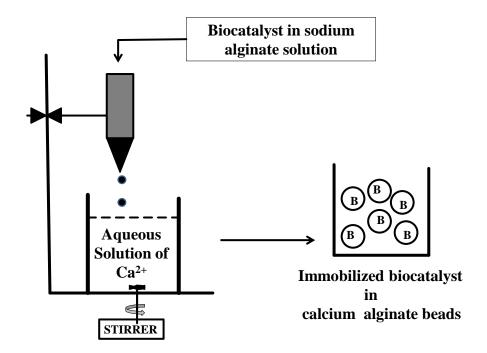
Figure 1: Sketch of encapsulation of a biocatalyst (enzyme, organelle or microbial cells) in calcium alginate beads.
