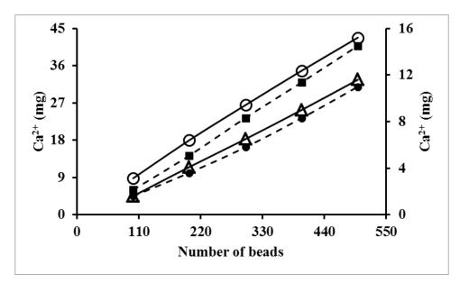
Figure 6: Number of beads in function of  $Ca^{2+}$  consumed for S1100 (10 g/L) polymerized at 30°C (dashed lines) and 40°C (solid lines) with  $CaCl_2$  0.1M [30°C: ( $\bullet$ ); 40°C: ( $\Delta$ )] and 0.4M [30°C: ( $\blacksquare$ ); 40°C: ( $\circ$ )].
