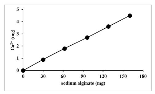
Figure 4: Correlation between sodium alginate and  $Ca^{2+}$  consumed. The gelation was carried out with SG800 (5 g/L) and 0.05M  $CaCl_2$  at  $30^{\circ}C$ .
