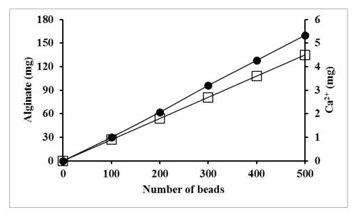
Figure 3: Variation of sodium alginate ( $\bullet$ ) and Ca<sup>2+</sup> ( $\square$ ) consumed in function of the number of beads obtained. The gelation was carried out with SG800 (5 g/L) and 0.05M CaCl<sub>2</sub> at 30°C.
