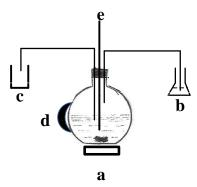
Figure 2: Sketch of the bench fermenter used for evaluating the fermentative capability of yeast cells. (a) Magnetic stirrer; (b) Flask containing the 0.5M sodium dithionite; (c) Sample harvester; (d) Heating jacket; (e) Thermometer.
